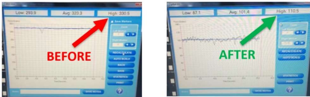
Figure 1. Photo image showing the strength values measured during the peeling of the stretch film on the pre-painted sheet
